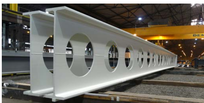
Final coating on fabricated girders
