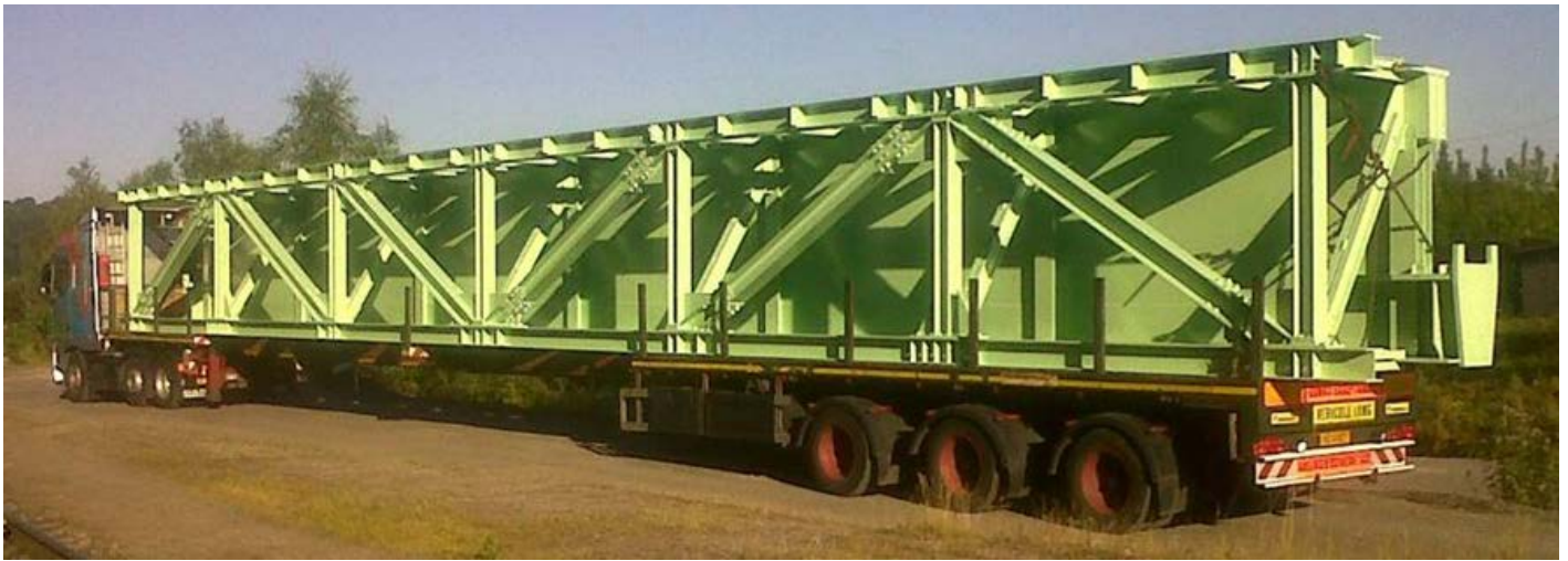
Truss structure for the runway crane in Belval still mill, Luxembourg
