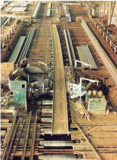
Finishing workshop - Cambering of bridge girders on the press.
