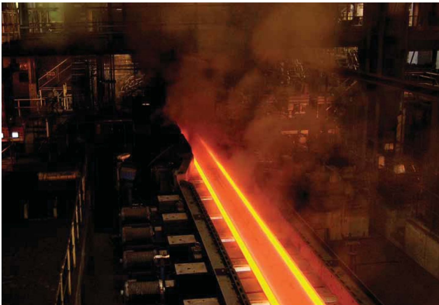
Rolling of a Histar beam in the rolling mill of Differdingen, Luxembourg
