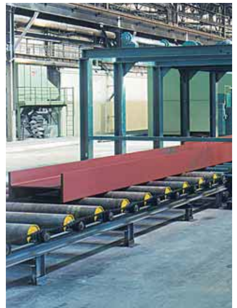
Automatic surface treatment equipment - Shot blasting and protective coating of beams.
