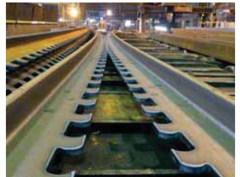
Separation of a PreCoBeam in the finishing shop of ArcelorMittal.
