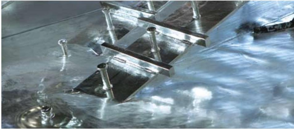
Nowadays, corrosion protection of steel car park structures is usually achieved by hot-dip galvanization. During this process, rust and mill scale are removed from the surface of the beam in a pickling bath before immersion during 5–10 minutes in the bath of liquid zinc at 450 °C. Typically, a 150–250 µm thick zinc layer is formed which will protect the steel surface against atmospheric corrosion.
