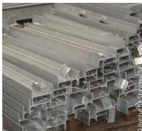
figure 9: Hot dip galvanized sections
