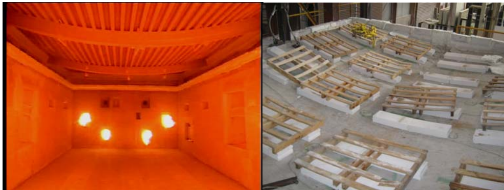
Figure 7.38 Tested floor during and after the fire
