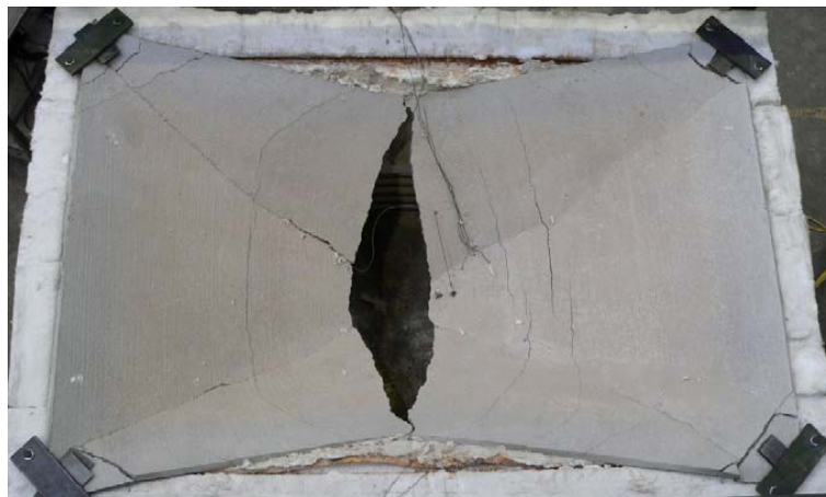
Figure 4.6 Mode of failure for test slabs at elevated temperatures
